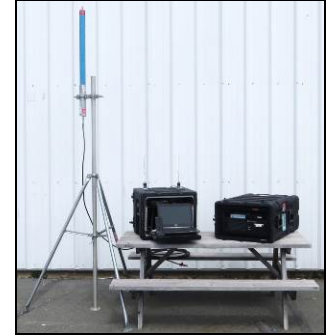
Tripod Antenna Unit
